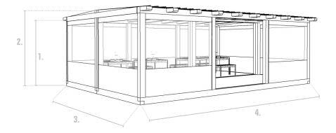
1. Side height: 2.22 m 2. Centre height: 2.50 m 3. Extendable per 2.50 m 4. Extendable per 2.50 m (min. 5m)
